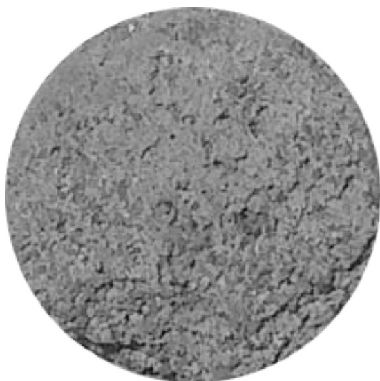
Fig. 3. The multi-hole structure of sample with NaCl after burning at or over than 1200 °C for 3 h.
