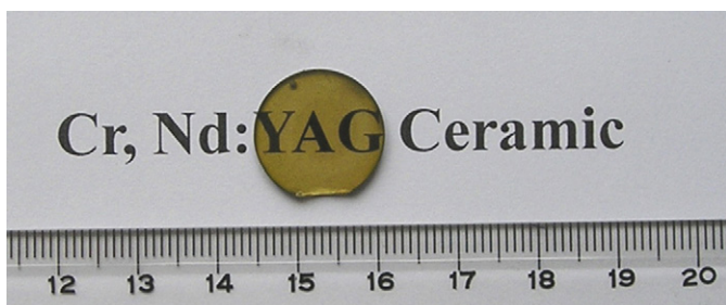
Fig. 6. Appearance of mirror-polished 0.1 at.% Cr, 1.0 at.% Nd:YAG transparent ceramics sintered at 1800 °C for 10 h.
