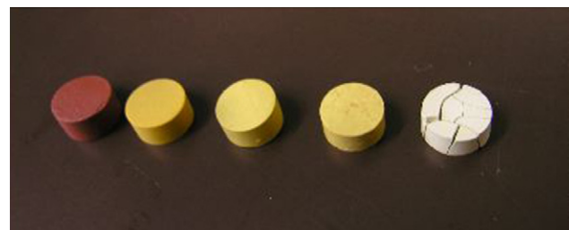
Fig. 2. Image of the fired samples. To the right there is the specimen obtained from PS alone showing extended fractures. To the left is set the sample made using CFA alone. In the middle are placed samples with intermediate compositions.
