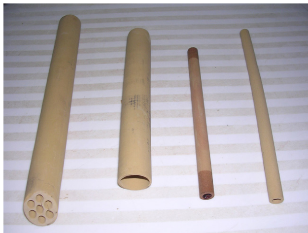
Fig. 3. A photograph of variety of configurations of porous ceramic supports.
