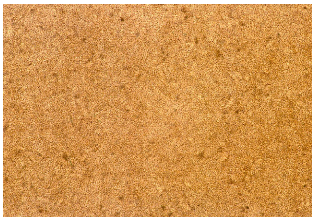
Fig. 8. Glass G1.5 Cr heat-treated at 680 °C, 1 h and then 950 °C, 1 h. Uniform very fine-grained texture, P.N. 400×.
