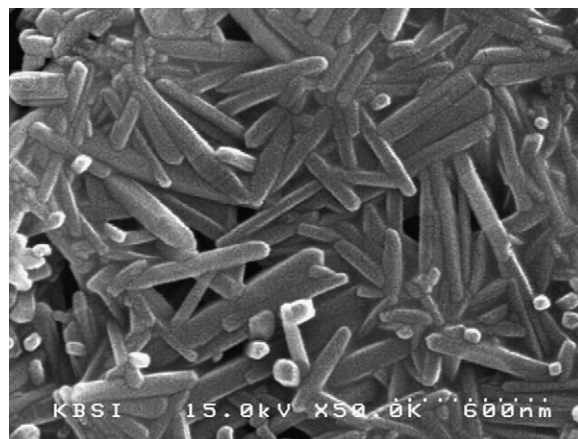
Fig. 2. SEM micrograph of the product obtained with an addition of 0.8 wt% \text{NaH}_2\text{PO}_4 \cdot 2\text{H}_2\text{O} ; fired at 1300^\circ\text{C} for 15 h; without chemically leaching.
