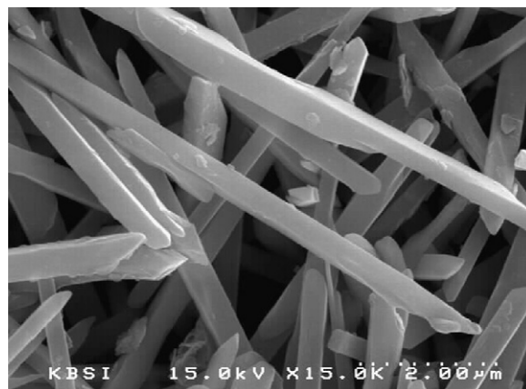
Fig. 8. SEM micrograph of the product obtained with an addition of 1.5 wt% \text{NaH}_2\text{PO}_4 \cdot 2\text{H}_2\text{O} ; fired at 1400 °C for 15 h; leached by 5 wt% HF solution at 50 °C for 3 h using microwave heating source.
