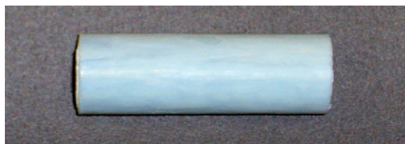
Fig. 6. Photograph of the glass-ceramics after crystallization under 1173 K for 15 h.
