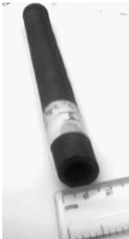
Fig. 7. Photograph of sintered LSM tube (contrast adjusted for clarity).
