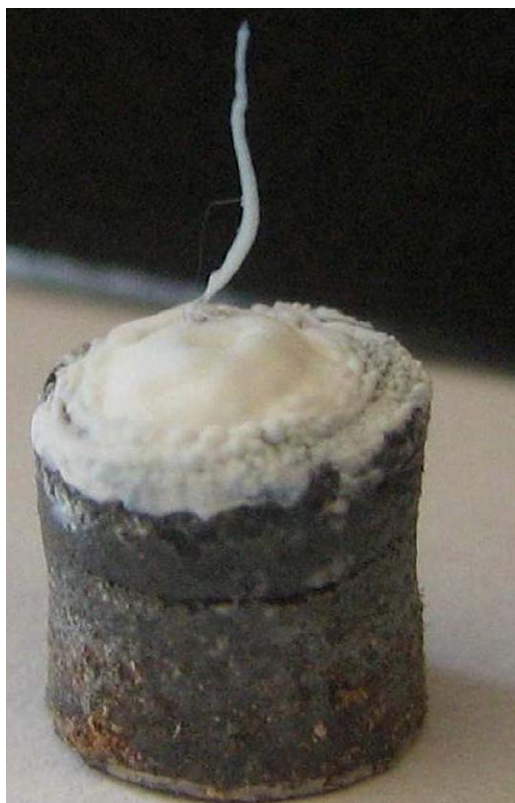
Fig. 4. Photograph of a SiC specimen laser-irradiated at P = 170 W.
