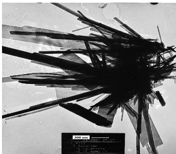
Fig. 4. The typical TEM micrograph of dandelion-like HAP.
