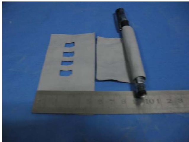
Fig. 6. Photograph of a green sheet wound on a column showing its flexibility, along with a strip showing holes made by punching.
