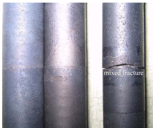
Fig. 4. Optical micrograph of the SiC joint samples (joined at 1200 °C).
