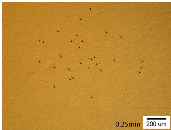
Fig. 3. Pseudo-plastic deformation pits in silicon nitride “A” that have been produced in 15 s of cavitation exposure. Optical microscope.
