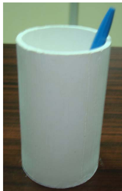
Fig. 2. A \text{MgAl}_2\text{O}_4 spinel crucible ( \sim 500\ \text{mL} capacity) consolidated by hydrolysis induced aqueous gelcasting (GCHAS) from a slurry containing 45 vol.% of T-MAS-5 + AlN (4.1 wt.%) powders.
