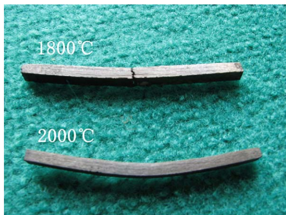
Fig. 4. The morphology of sample C/SiC–ZrB 2 (ZB-40) composites after flexural strength tests at high temperatures.
