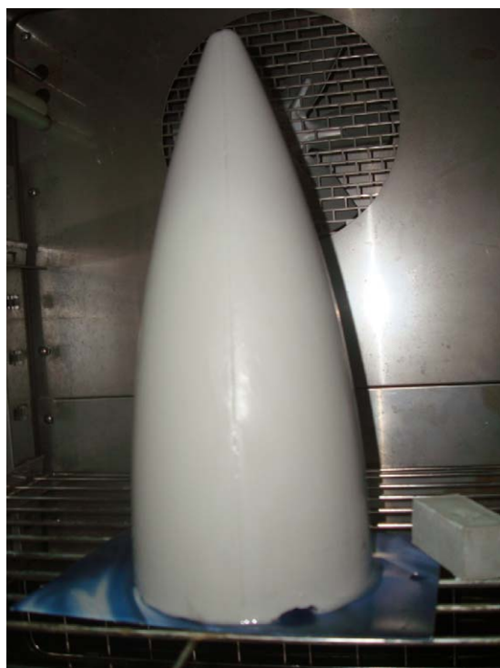
Fig. 1. A green radome shape (about 290 mm height and 125 mm base diameter) consolidated by hydrolysis induced aqueous gelcasting (GCHAS) of a suspension containing 50 vol.% of alumina + 4 wt.% AlN in a split-type Teflon lined aluminium mould.
