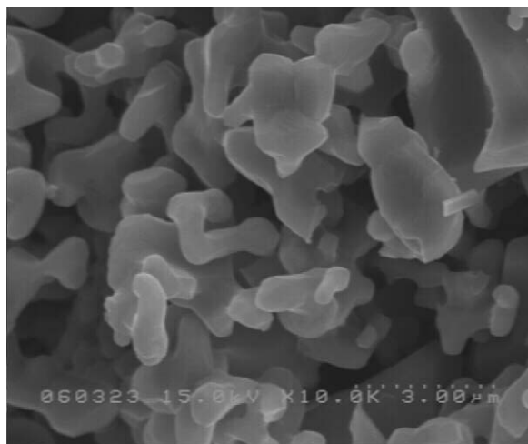
Fig. 1. SEM for the copper ferrite powder ( \text{CuFe}_2\text{O}_4 ) annealed at 800 °C for 1 h.
