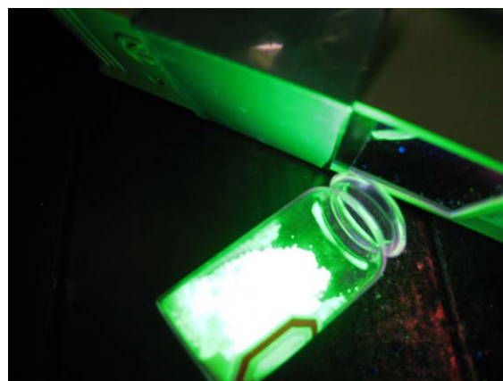
Fig. 6. Photograph for the green light emission of calcined \text{Zn}_2\text{SiO}_4:\text{Mn}^{2+} phosphors.
