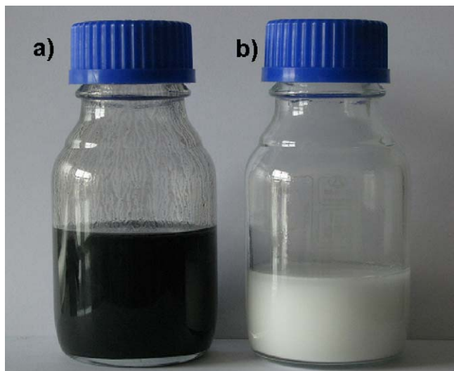
Fig. 8. Photo images of MWCNT/boehmite mixture (a) and alpha alumina stable suspension with a 3 wt.% solid-loading (b).
