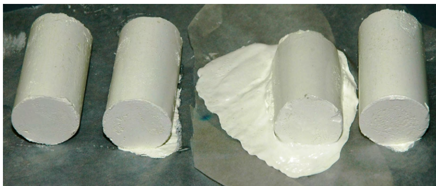
Fig. 8. Photograph showing the relative stability of the gels repaired at various MgO concentrations against the oscillatory stresses. Bodies after vibration test (from left) 0.07 wt% MgO, 0.05 wt% MgO, 0.04 wt% MgO, 0.04 wt% MgO (before vibration test).
