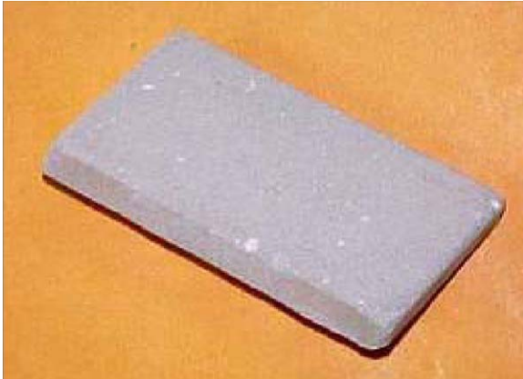
Fig. 6. Green body obtained by uniaxial pressing of ash mixed with powdered cullet glass (dimensions: 70 mm × 40 mm × 10 mm).
