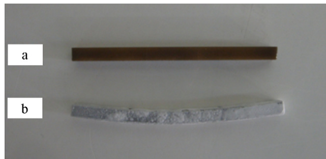
Fig. 7. Visual observation of (a) as-sintered and (b) crept specimens.
