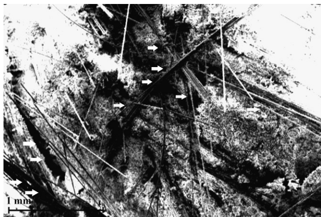
Fig. 9. The SEM micrograph of the fractured composite sample containing 25% BGF after compression test.
