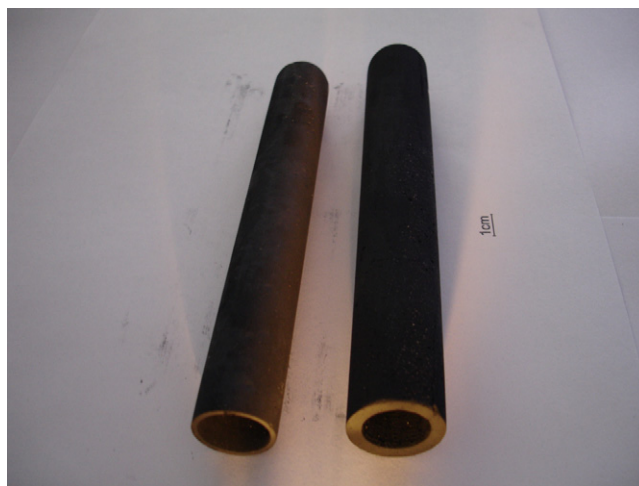
Fig. 4. Typical slip cast LSM tubes sintered at 1400^\circ\text{C} .
