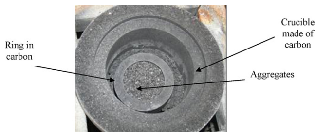
Fig. 2. Detail of the corrosion apparatus: view of grains in the carbon crucible.
