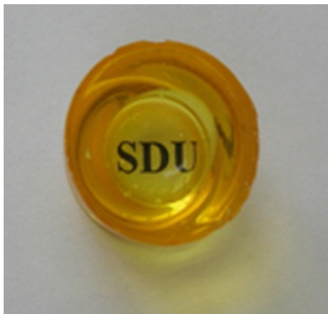
Fig. 2. Optical photograph of zirconia xerogel after aging and drying at 60 °C for 100 h.
