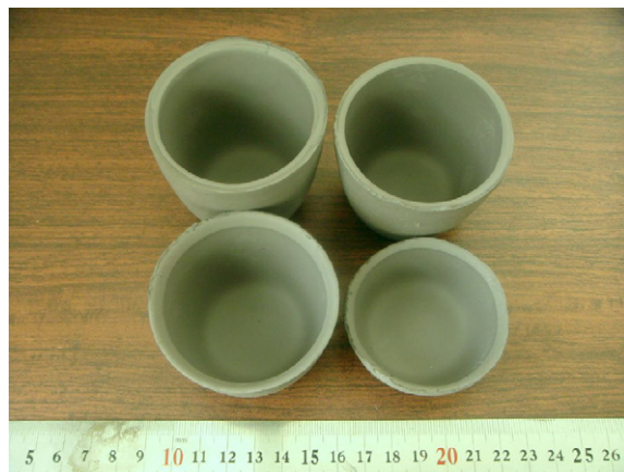
Fig. 5. Photo of green crucible bodies prepared by 40 wt% solid load slurries.
