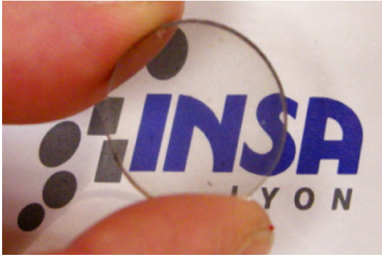
Fig. 5. Visual appearance of the S30CR spinel sample sintered up to 1300 °C (2.3 mm thickness) (the left sample is 30 mm above the printed text).
