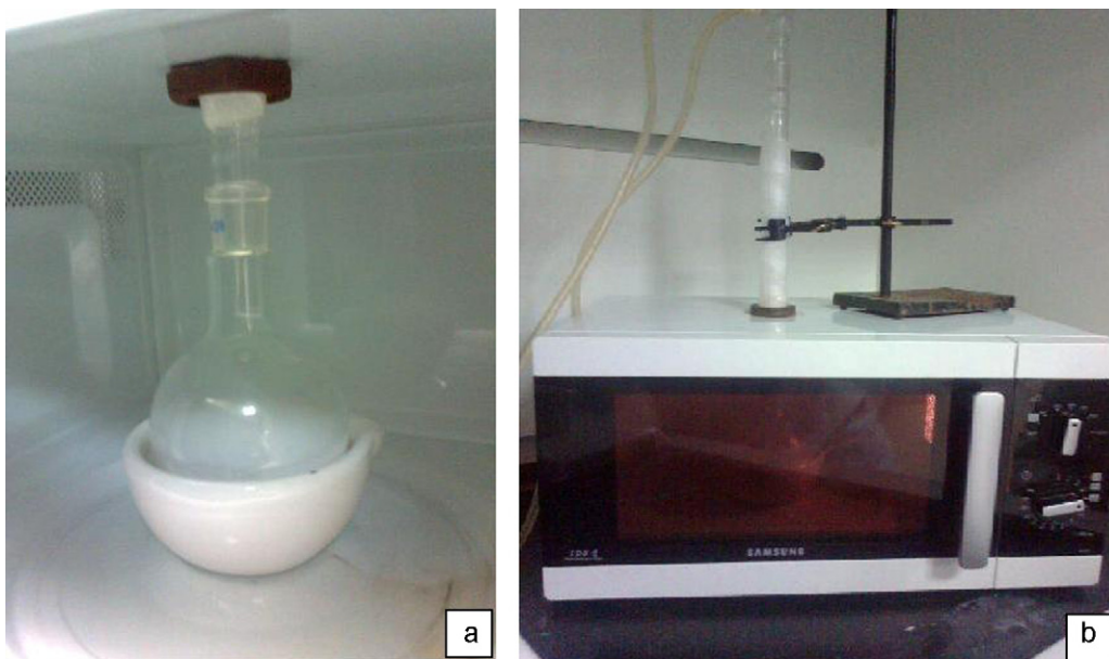
Fig. 1. Experimental set up for microwave assisted synthesis of HA in our laboratory: (a) interior view and (b) exterior view.
