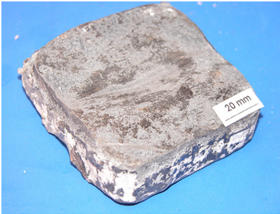
Fig. 2. \text{SiC}_p/\text{Al}_2\text{O}_3 composite by directed metal oxidation process ( 70 \times 70 \times 20 , in mm).
