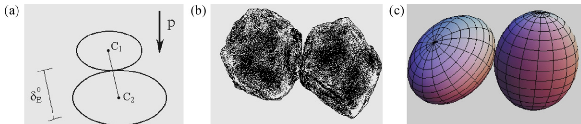
Fig. 3. (a) Ellipsoidal approximation, (b) and (c) two grains in contact according to ellipsoid–ellipsoid model.
