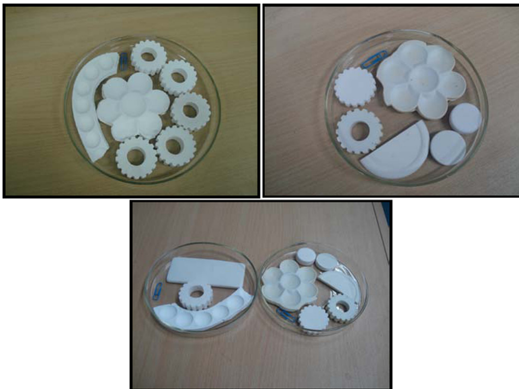
Fig. 10. Photographs of Titania gelcast components.
