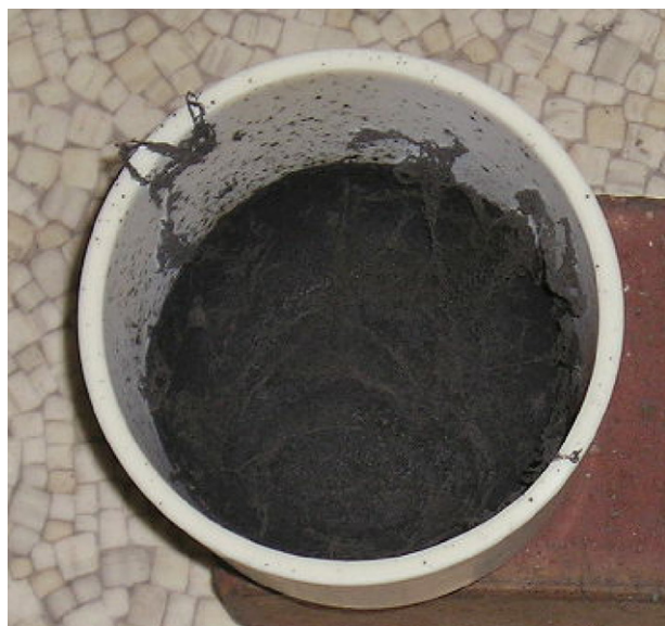
Fig. 1. Photograph of \text{LiNiO}_2 precursor after combustion reaction at 400^\circ\text{C} .
