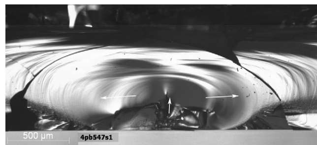
Fig. 8. Sectional view for the fracture surface of cracked coated sample tested in four-point bending. The figure shows that crack origin is nearly the middle of the median crack.
