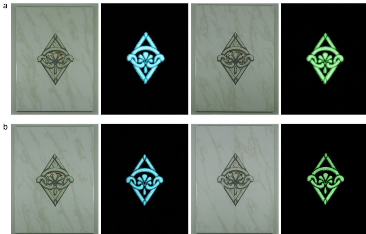
Fig. 17. The final appearances of decorated, glazed wall tiles in the day light and the dark. Decors contain 10% BG and YG pigments and single fast-fired at 920 °C (a) and 980 °C (b) in Vitra Karo Inc.
