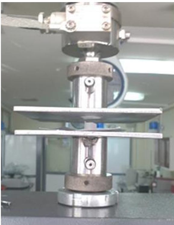
Fig. 5. The uniaxial compression test machine with its two steel plates.
