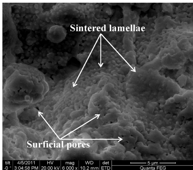
Fig. 20. High magnification image of top surface of YSZ duplex coating after thermal cycling.
