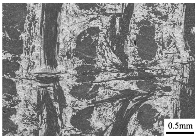
Fig. 4. Cross-section of C/C–SiC–ZrC composites fabricated at 1800 °C for 30 min.
