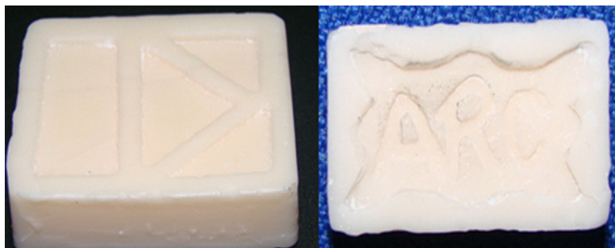
Fig. 9. Sintered thermal gel cast samples after milling and drilling.
