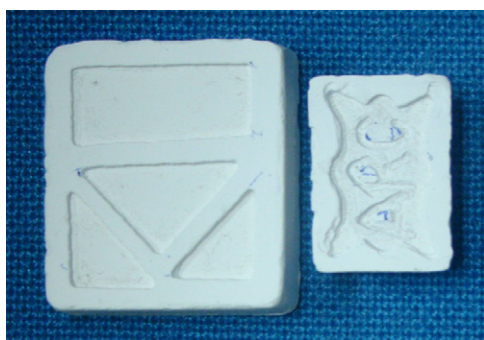
Fig. 8. Green thermal gel cast samples after milling and drilling.
