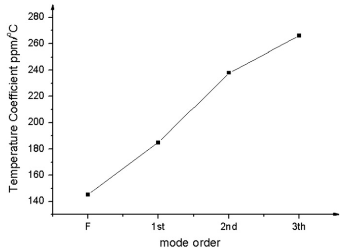
Fig. 7. The temperature coefficient of resonant frequency (TCF) of the piezoelectric ceramic disk versus mode order.
