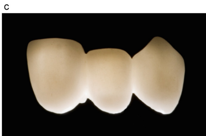
Fig. 4. Photographs of (a) self-colored zirconia framework, (b) all-ceramic prosthesis, and (c) translucency of the prosthesis.
