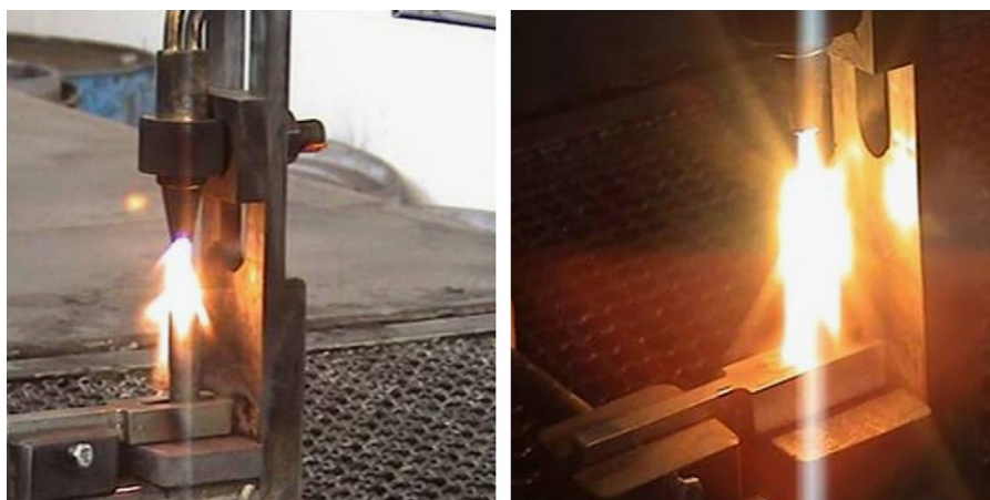
Fig. 2. Oxyacetylene ablation facility operating at approximately 2000 °C.
