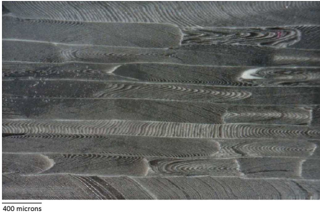
Fig. 9. Optical cross section view of an SG-B four-point bend bar specimen. Cross section was obtained by an inclined cut at 60^\circ . Rectangular cells representing cross section views of the first order lamellae are seen in this cross section. Also visible are the second order layers within each rectangular first order cell.
