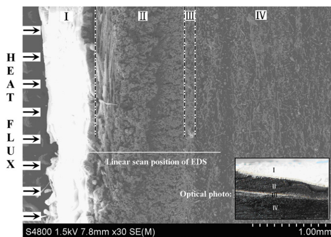
Fig. 1. Longitudinal profile image of the silicone rubber composite after ablation.
