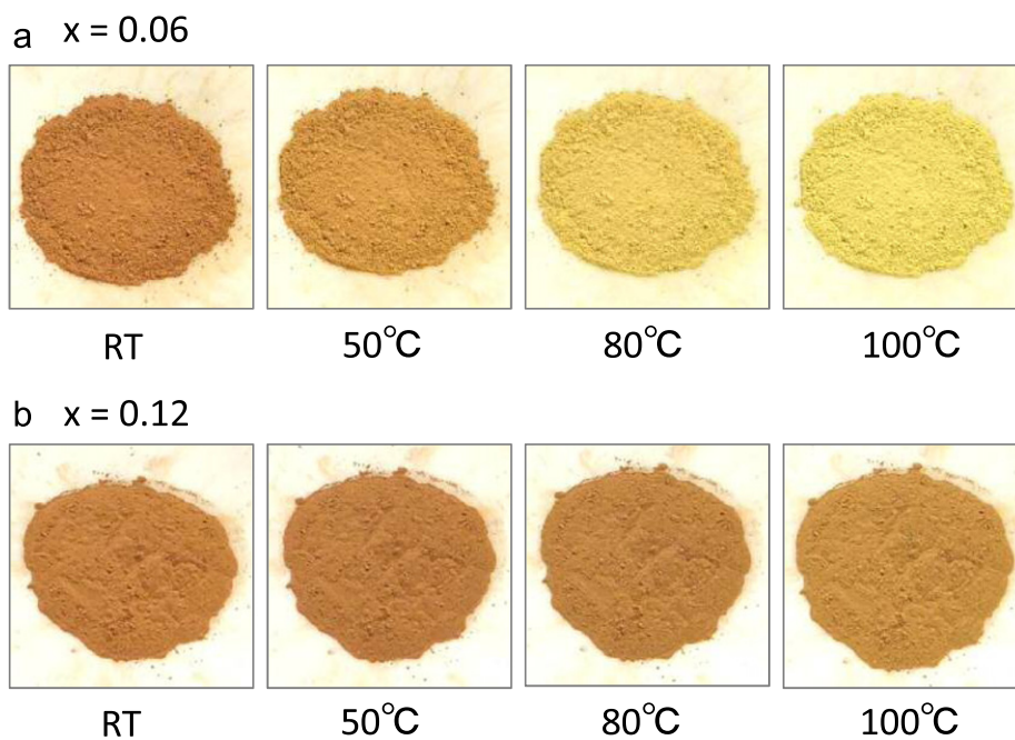
Fig. 8. Change in color of (a) \text{CuMo}_{1-x}\text{W}_x\text{O}_4 ( x=0.06 ) and (b) \text{CuMo}_{1-x}\text{W}_x\text{O}_4 ( x=0.12 ) powders in the range from RT to 100 °C.
