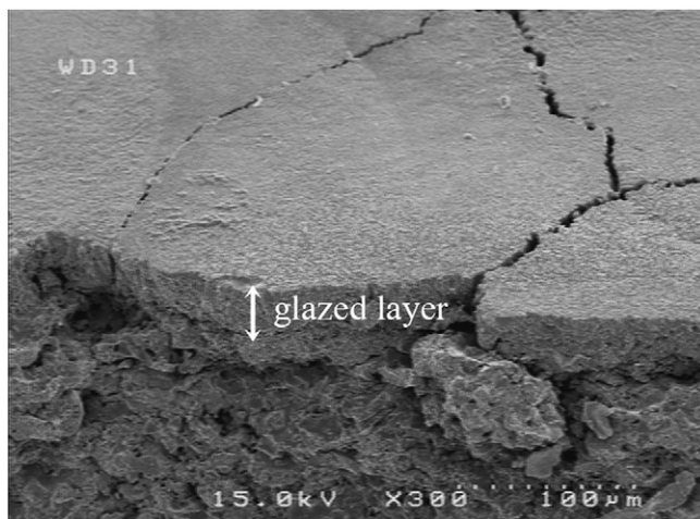
Fig. 8. FESEM micrograph of fractured cross section of laser glazed coating.
