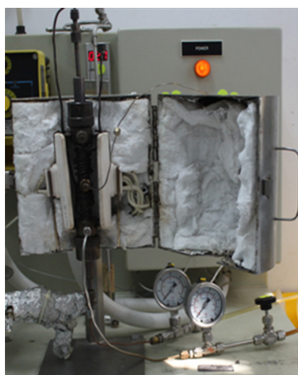
Fig. 1. Image and schematic of the Pd–alumina MR system.
