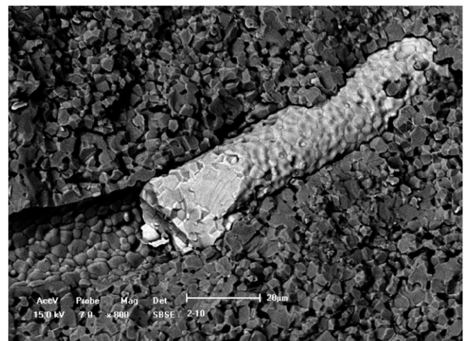
Fig. 12. A typical interface micrograph of \text{ZrO}_{2(t)}/\text{NiFe}_2\text{O}_4 composites.
