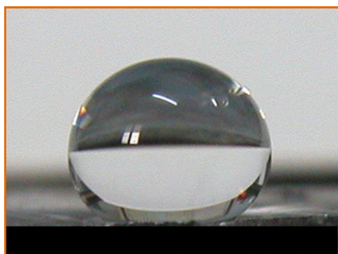
Fig. 6. WCA image of the hexagonal Cu-ZnO nano-funnel tube film grown on zinc substrate.
