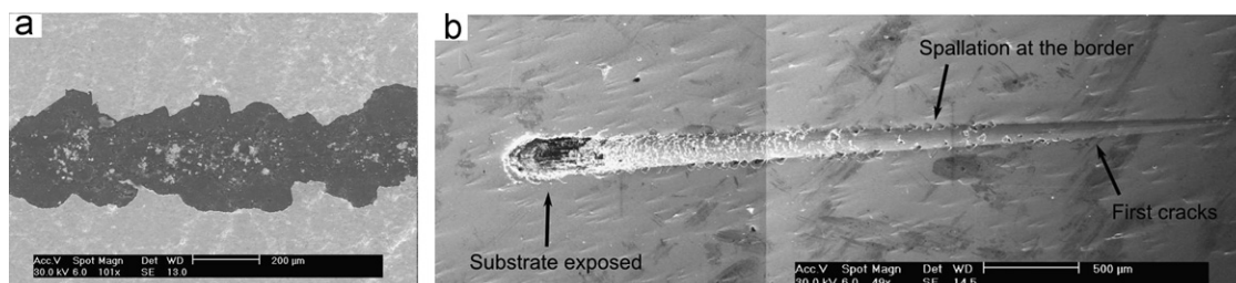
Fig. 9. SEM micrograph of the scratch track (a) on HD graphite and (b) on Nb sample.
